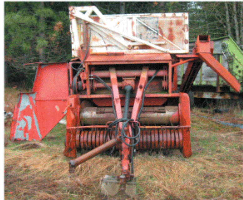
Bean Combine, front (production capacity 75 tons / day - auto hulling and cleaning, on board)
